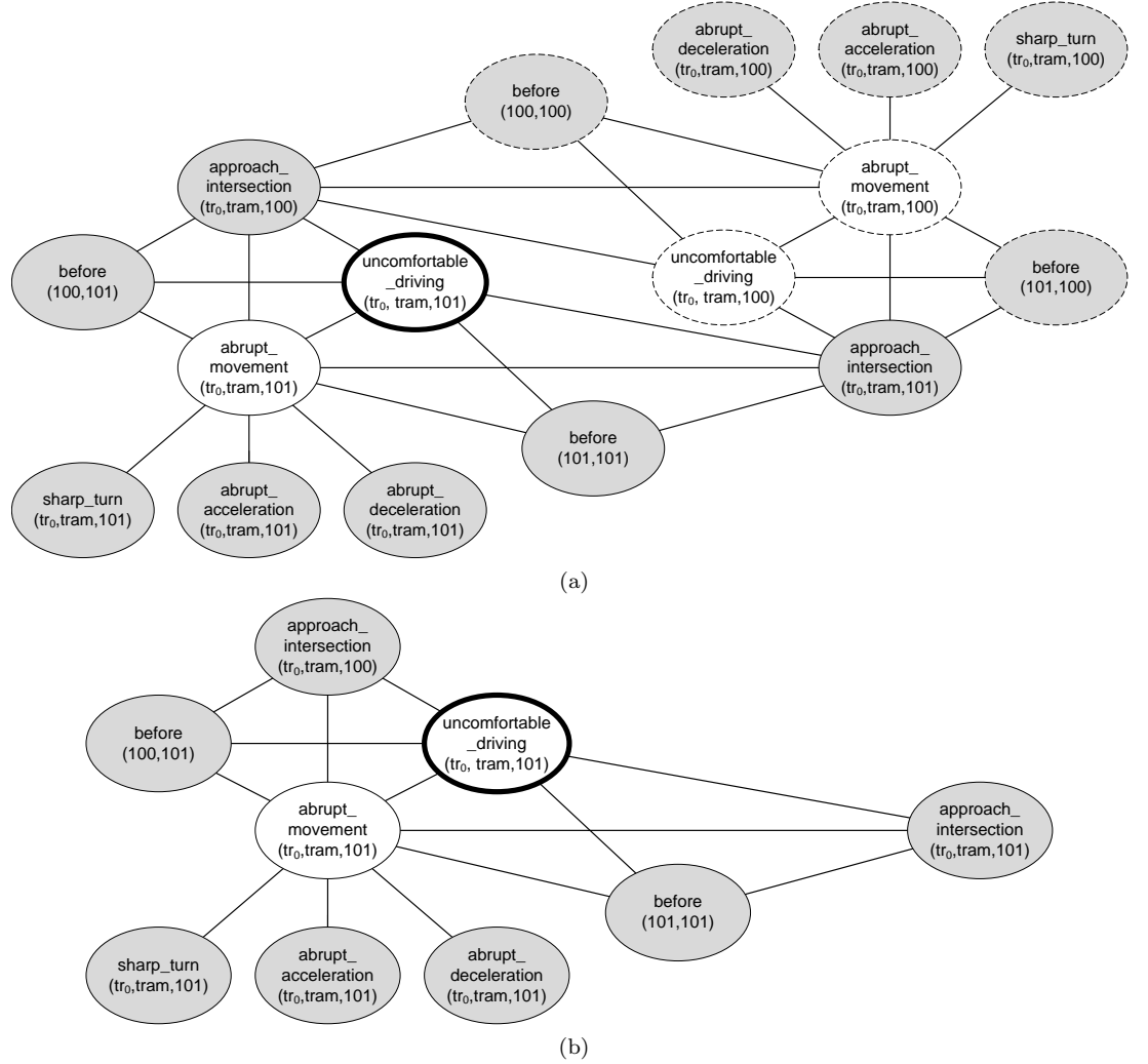
Fig. 9: (a) Complete Ground Markov Network. (b) Ground Markov Network Reduced for Event Recognition. Nodes with a thick line represent query variables, shaded nodes represent variables with known truth values, and nodes with a dashed line represent variables which can be safely removed.
